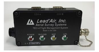
The TECI-4 likewise performs many other tasks: exposing the details of the mission and the photo position on film (RC30, RMK TOP, etc.); automatically controlling all the camera functions, v/h, FMC, drift, etc. (with the necessary optional equipment) as well as interfacing with most camera mounts and stabilized platforms (*Track'Air Steadytrack,* PAV 30, GSM 3000, TAS, etc.).
